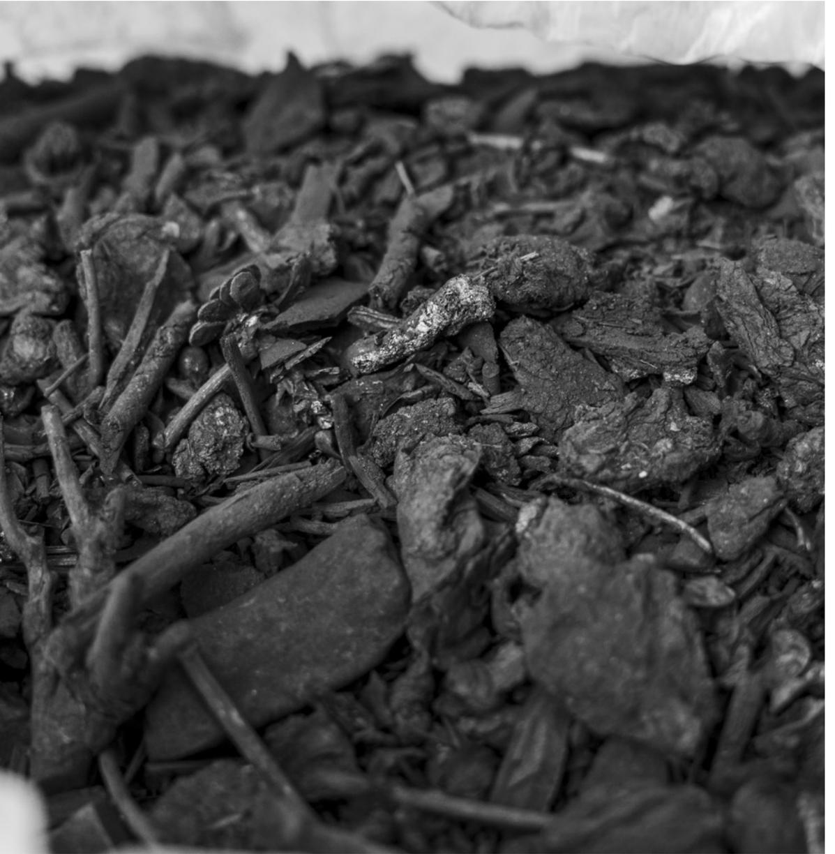
Problematic wastestreams: Recarbonization of screen overflow (made in the laboratory)
