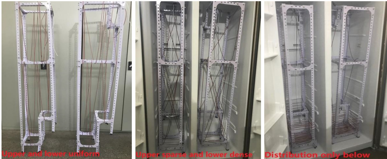
Fig. 4. Distribution modes of electric heating wire.
